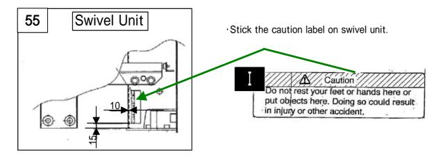
Please make sure the Unit swivels properly after finishing installation.
