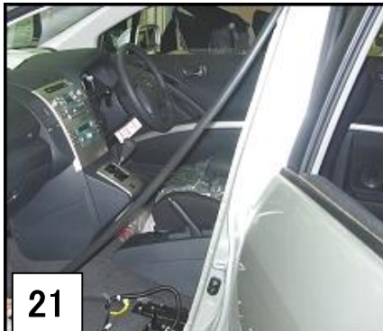
6. Remove the glove compartment.
