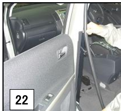
4. Remove the rear weather strips.
