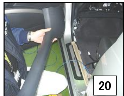
5. Remove the B pillar lower trim.
