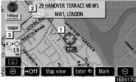
Use the scroll feature to move the desired point to the centre of the screen for looking at a point on the map that is different from the current position of the vehicle.
