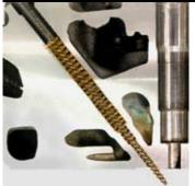
Remove the glow plugs. Clean the glow plug shafts with stepped brass wire brush p/n PZ 485 904 9026.
