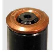
Get a new sealing ring and place it on the extraction claw in order to adjust the grip depth. The length of the claw can be changed by turning. The claw is optimally adjusted when the collar protrudes minimally over the sealing ring. If the collar protrudes too much, the extractor will jam in the bore of the nozzle and can not grip the sealing ring. Also is there a risk of damaging the cylinder head. If the claw is not adjusted enough, then the extractor will not grip the sealing ring.
