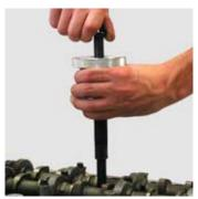
Place the sealing ring extractor p/n PZ471 6039070 in the shaft with the slide hammer p/n PZ 485 903 90750 screwed on and knock, with feeling, the claw into the hole of the sealing ring. Remove the slide hammer.
