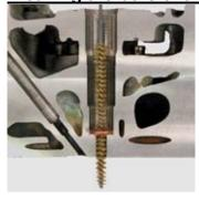
Remove the dirt and debris from bore of the nozzle with the brass wire brush p/n PZ 485 904 9025
