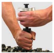
Screw the slide hammer on the sealing ring extractor and knock with feeling the copper seal out of the injector shaft .
