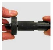
The knurled actuator of the sealing ring extractor must be freely movable and should have some play from the knurled pipe.
