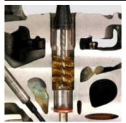
Measure the diameter of the removed injector and select the appropriate brass brush:
