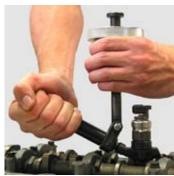
In very severe cases the injector can be removed with the pivot adapter p/n PZ 485 903 8440 and the slide hammer p/n PZ 485 603 90750. Remove the O-ring, slide the pivot adapter p/n PZ 485 903 8440 on the handle and return the O-ring in the groove on the handle. Screw the handle on the diesel connector and the slide hammer on the pivot adapter. Knock by simultaneously rotating and striking the injector from the shaft.
