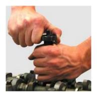
Grip the sealing ring by turning the knurled actuator and holding the knurled pipe.
