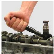
If injector can not be removed easily, then it is possible with the handle p/n PZ 485 903 8438 for outer thread or handle p/n PZ 485 903 8437 for inner thread screwed onto the diesel connection, through turning and pulling to remove the injector from the shaft.
