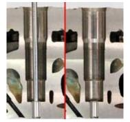
Place the sealing plug by means of the setting tool in the injector shaft and remove the setting tool.
