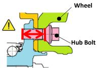
WARNING: Using a bolt that is too short or too long may prevent the proper tightening torque from being achieved.
