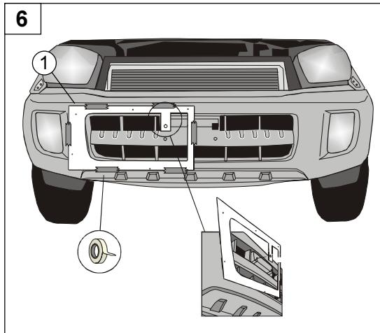
• Fit the drilling template (1) to the bumper by adhesive tape and make sure it is aligned with the license plate fixation hole, as shown in figure 6.
