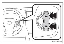
By pressing the telephone switch, you can receive a call or hang up without taking your hands off the steering wheel.
