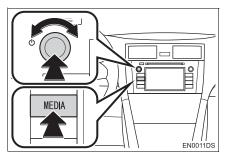
"MEDIA" button: Press this button to display screen buttons for the audio system.
