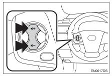
By pressing the volume switch, you can adjust the volume.
