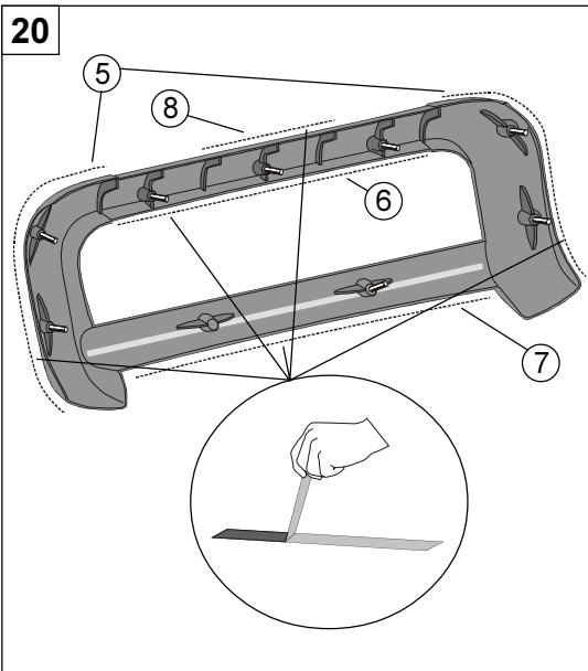
• Remove the protective film of the textiles (5), (6), (7) and of the transparent film (8). The corresponding position is shown in figure 20.
