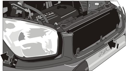
• Fit the metal frame and push inwards, as shown in figure 24.
