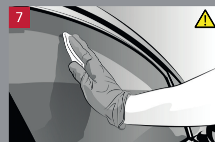
Apply Toyota ProTect to side windows in the same way.
