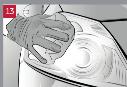
Buff carefully for a smooth, protected finish using the dry grey cloth from the kit.
