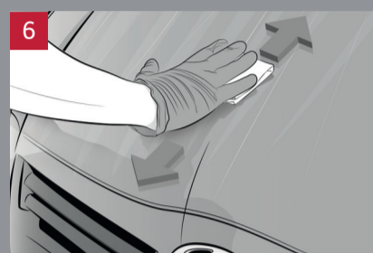
Wipe Toyota ProTect onto panels in straight lines.
