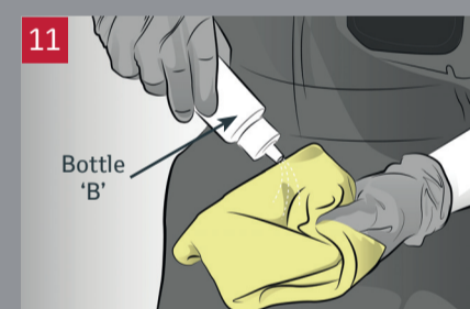
Dampen the yellow cloth, shake the Hardener bottle 'B' and add to the cloth.
