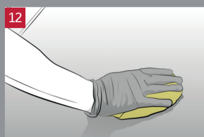
Apply Hardener to all previously treated bodywork and side windows.
