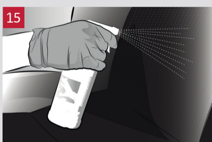
Spray evenly at a distance of 20-25 cm. Double application on driver's seat.
